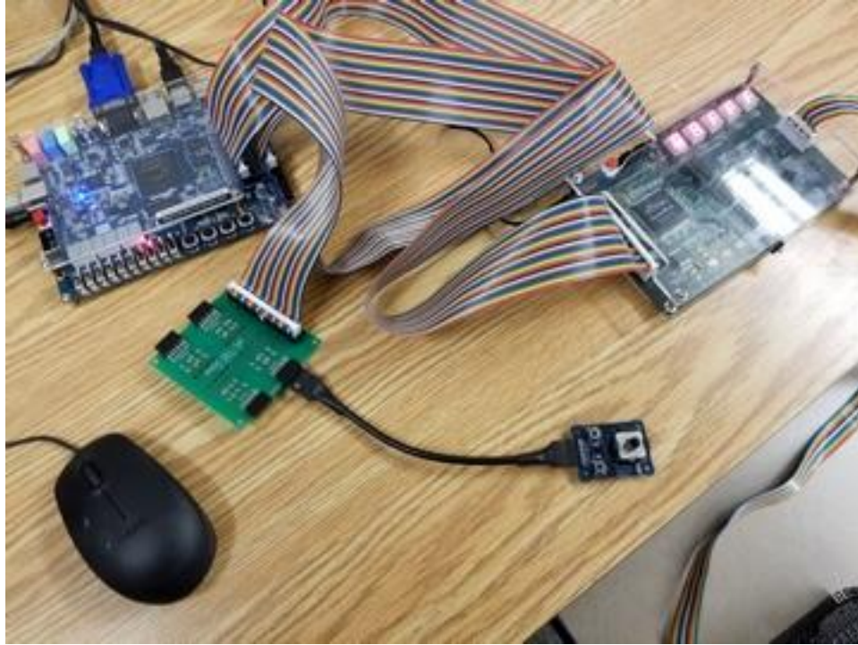
Figure 7 -closer view PMOD board is connected to GPIO 0 and Lego controller connected to GPIO 1
