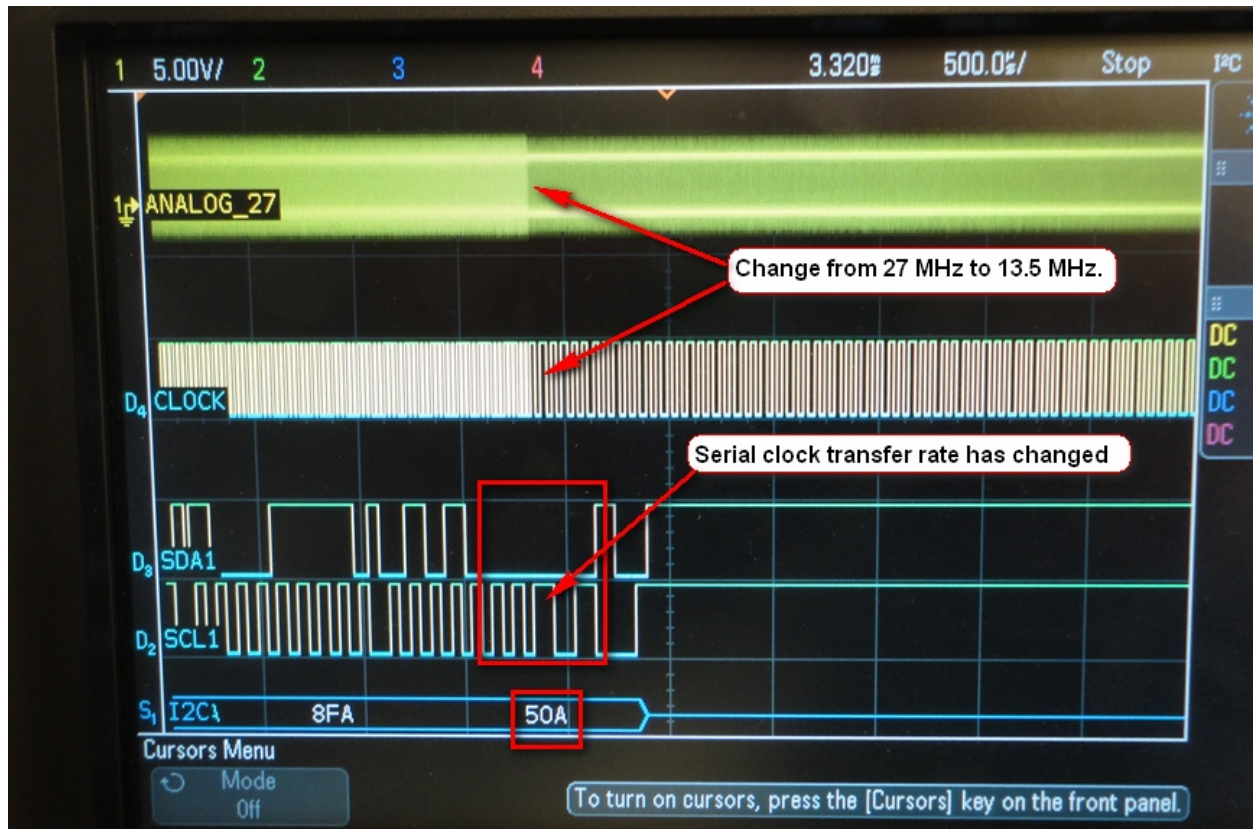
Figure 22 – clk_27 frequency changed from 27 MHz to 13.5 MHz
