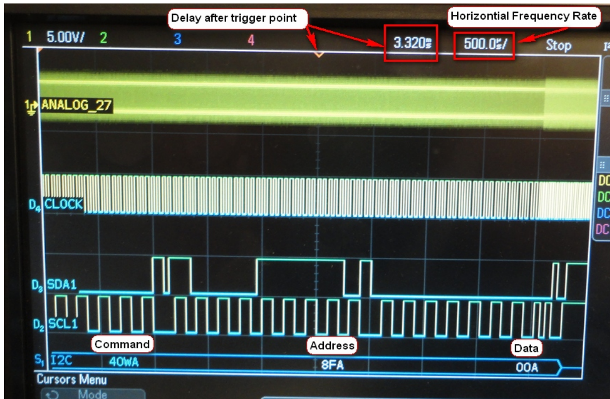
Figure 24–The default frequency changes from 13.5 MHz to 27 MHz
